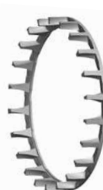
Fig. 7. YMD Split, machined-brass, land-riding, finger-type cage.
