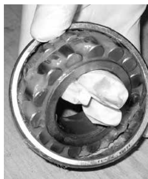
Fig. 21. Grease can easily be packed by hand.
